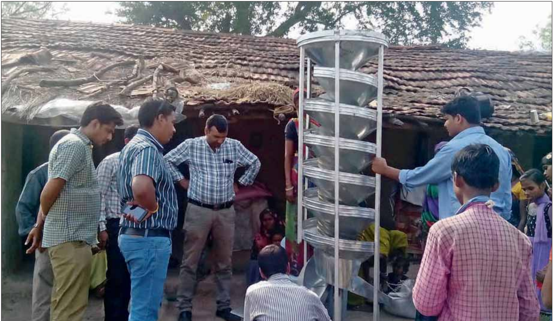
A low cost soybean grader given to women enterprise group as part of farm tools and equipment library in Mhow block MP
