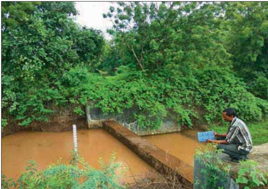
Bhujal jankar takes daily water level reading to study ground water recharge rate in watershed area
